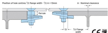
Material: Malleable iron, zinc plated / hot dip galvanised. Stainless steel grade 316.
